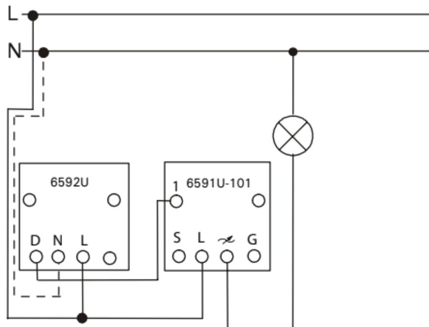
5 extension units maximum can be operated in parallel.
