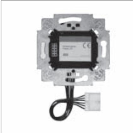
The binary input/sensor is a flush-mounted device and is used for the potential-free connection of conventional push buttons and switches. The device is suitable for insertion in a 60 mm flush-type box.
